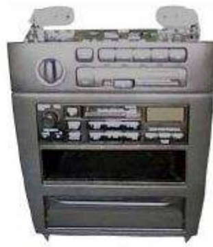
Photo of the radio/air conditioner assembly after being removed from the vehicle.
