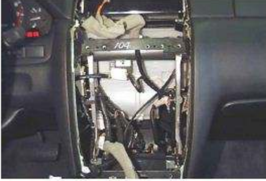
Photo after radio/air conditioner assembly has been completely removed from the dash.
