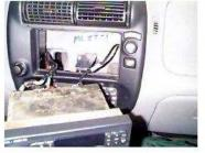
STEP 1: The Ford radio is snapped into the vehicles dash. With the proper tool, known as Ford radio removal keys, the Ford radio can be pulled forward out of the dash. A clothes hanger can be used instead of actual Ford radio removal keys. Cut the clothes hanger and bend 2 pieces in a 'U' shape
